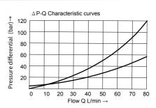
ΔP-Q- characteristic curve, flowing via one-way valve B to A.
